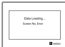
Before starting communications with the PLC, check the data in [Read Area] "n + 2" and confirm that the screen number to be displayed at first is specified.
