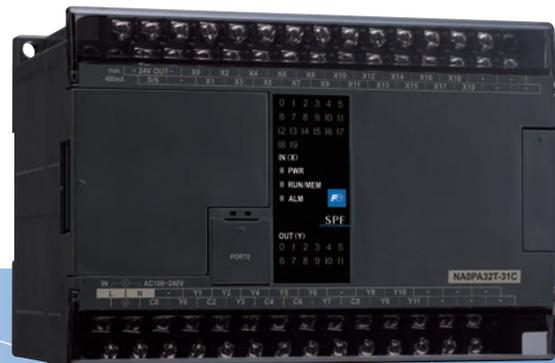
MICREX-SX SPF Plus provides advanced motion control, such as synchronous and circular interpolation controls.
