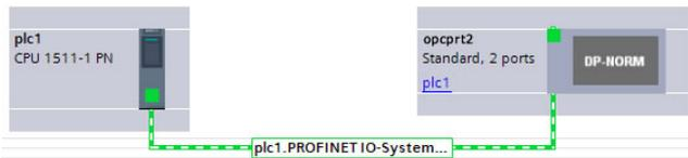
Figure 48: PROFINET IO System
